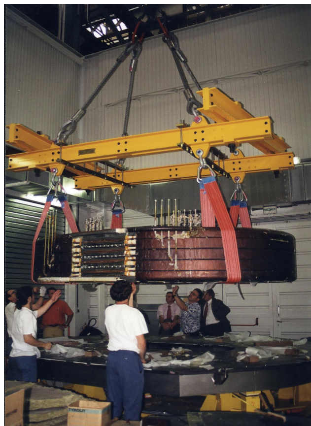
Fig. 4: The impregnated winding pack consisting of five double-pancake modules
