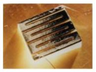
The sensitive element in QMC Instruments' detector is a small slice of ultra-pure Indium Antimonide which is cut in a zigzag pattern and mounted in a liquid helium cryostat at -269 C. Low thermal conductivity wires carry the tiny electrical signals to external room temperature electronics.
