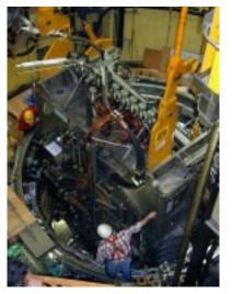
The TFMC during lifting procedure in the TOSKA vacuum vessel
