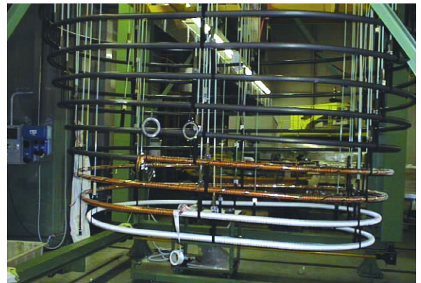
Ansaldo - DP1; lower pancake inserted, transfer of upper pancake on going. Genoa, 6 April 98.
