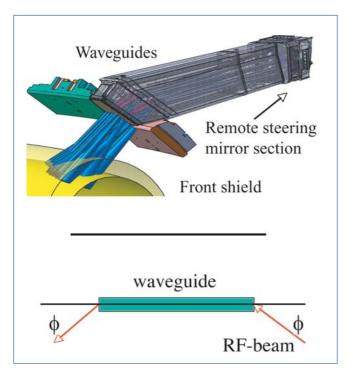
Fig. 1: ITER upper-port for ECRH-launcher
