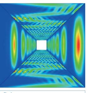
Fig. 2: Calculated wave field pattern at the inner RSL-wave guide walls. The zig-zag like propagation of the wave along the wave guide is clearly seen. The calculations were performed at IPF Stuttgart.
